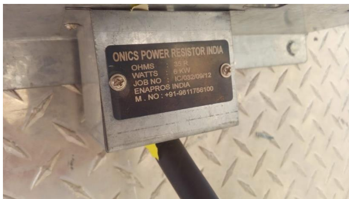
Figure 1: Name Plate of Load Resistor
