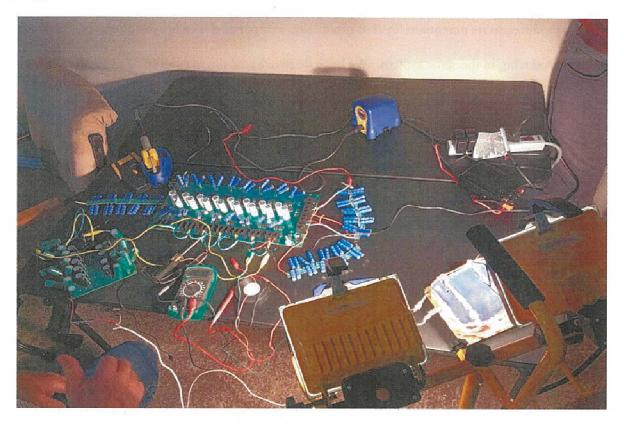
The solar PV cells are connected, not in a parallel, nor are they connected in the usual serial format, each solar cell is completely independent and it is controlled by what we call a voltage control board, which makes it so that each solar cell is completely independent from every other solar cell. In the traditional solar cells that are being used today, they are connected
