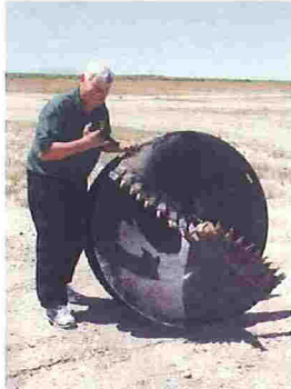
Installation: The drill head used for making holes in the ground for the towers to be set.
