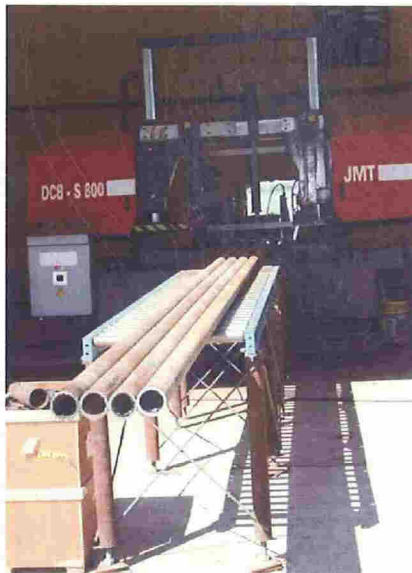
Manufacturing: The pipe cutter has been programmed and an automatic feeding system has been added to increase productivity.
