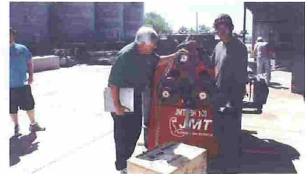
Manufacturing: This automated machine is specialized to bend pipes to make large rings that house our solar lenses.
