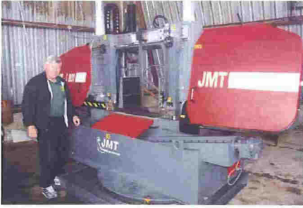
Manufacturing: New robust pipe cutter delivered and installed can cut through 5 pipes at a time.
