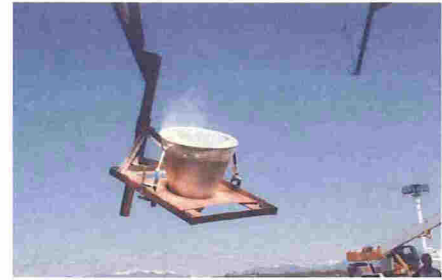
Field Testing: By adding the parabolic heat concentrator, we were able to achieve focal point temperatures nearing 3,000 degrees F.
