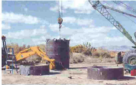
Biomass Testing: The Burner includes a cyclone in the upper chamber that burns off all toxins. The only emission is CO2. It doesn't need a boiler and works with our pipe-less heat exchanger.
