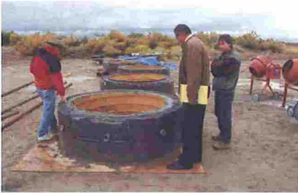
Biomass Testing: This R&D Biomass Burner was built to work in tandem with our solar towers for 24-hour operation with power generation and water distillation.
