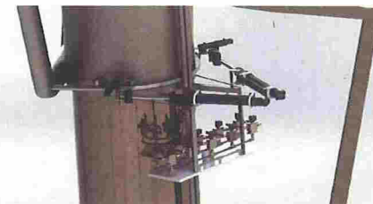
Manufacturing: Completed 3D CAD design for our hydraulic dual-axis solar tracking system.
