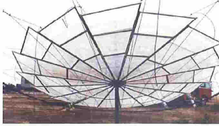
Solar Disc Design: Bottom view of the original solar disc design.
