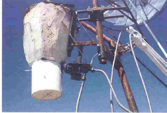
Installation: Mounted insulated heat concentrator with protected heat collector.
