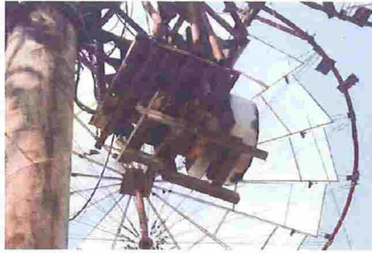
Field Testing: The tower-mounted concept worked but did not end up saving any time or money on construction so we went back to the original in-series model.
